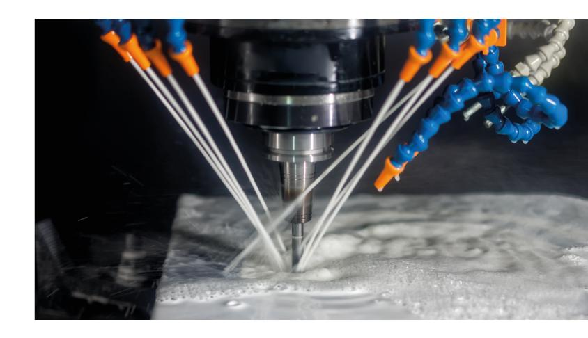
The universality of Safecut M 145 NT is also demonstrated by the different materials that can be worked using this emulsion. For instance, it is suitable for all yellow metals, aluminium, steel and alloys, stainless steel and even titanium.
